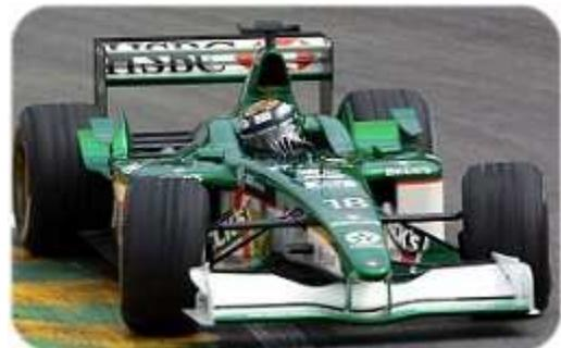
Each part of the car is made from exotic composite materials for maximum performance and minimum weight. Even though the rules of FIA (Federation Internationale de l'Automobile) state that each car, including driver, must not weigh less than 600kg, reducing the weight of the car's components allows redistribution of the weight enabling the car to go through turns quicker.
